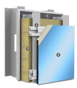
Structural Back-up Wall (by others): Steel or wood frame with glass mat gypsum sheathing in compliance with ASTM C1177, code compliant OSB or plywood sheathing, concrete or concrete masonry, existing structurally sound, uncoated brick or other masonry wall construction.
