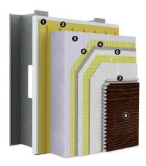
Substrate: Glass Mat Gypsum sheathing in compliance with ASTM C 1177, Exterior or Exposure I wood-based sheathing (plywood or OSB), cement board in compliance with ASTM C1325, or code compliant concrete, concrete masonry or portland cement plaster, existing strucuturally sound, uncoated brick or other masonry wall construction.
