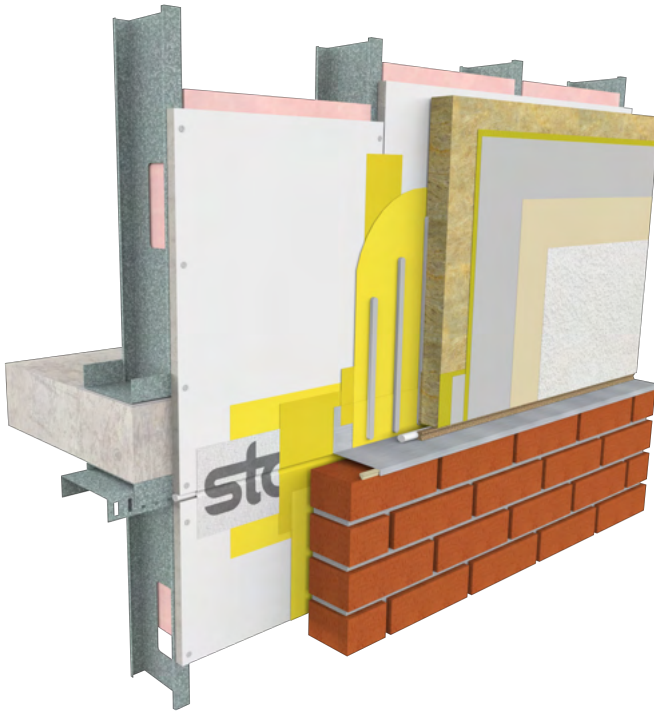
Typical working joints in StoTherm ci Mineral at floorline deflection joint and at dissimilar construction
